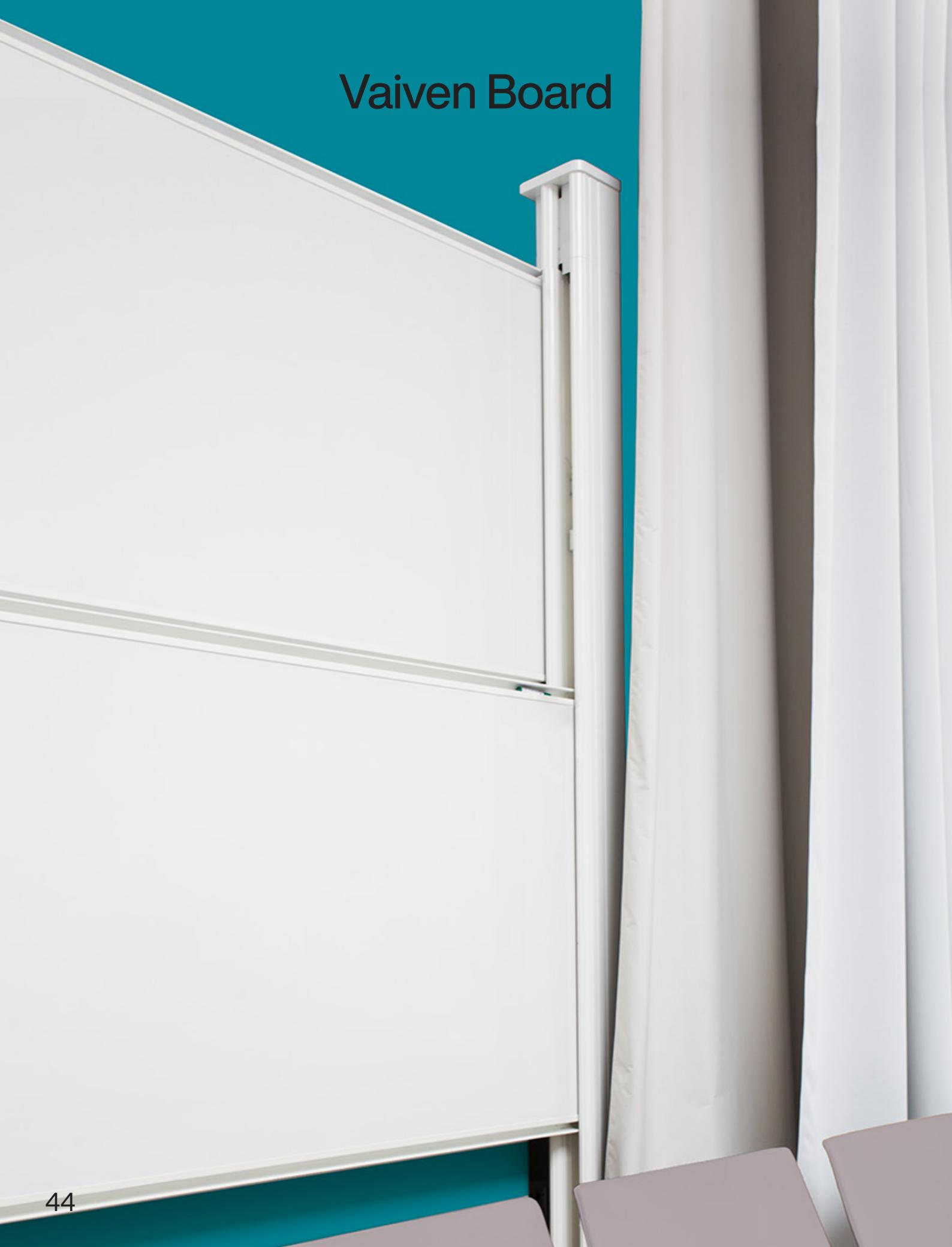
Vaivén blackboard made of white vitrified steel for dry erase markers or green for chalk. Aluminum structure wall or floor mounted. The boards slide easily and are guided in the profiles by nylon bearings. Ideal for schools, universities, amphitheaters, auditoriums... The two blackboards are offset one with the other. When one goes up the other goes down and vice versa.
